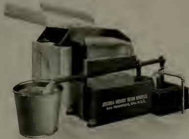
Automatic Tailings Sampler as Used in Sampling Tailings from the Battery After Passing Through an Amalgam Trap
